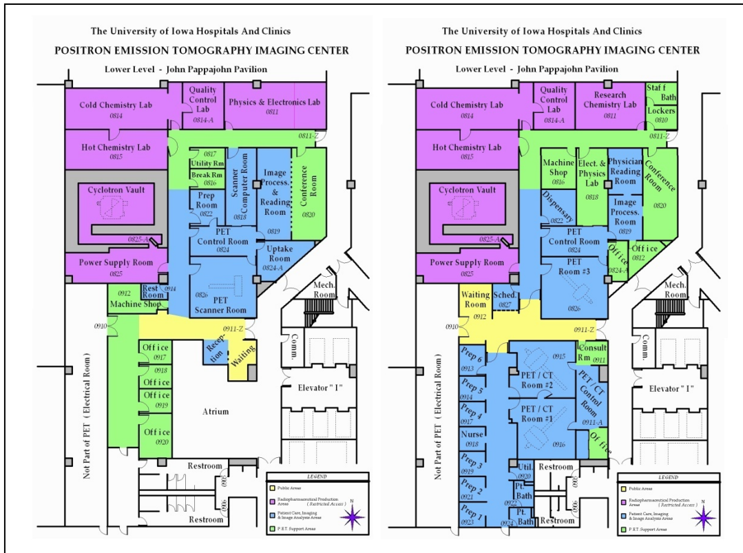
Figure 1. The University of Iowa Hospitals and Clinics, Positron Emission Tomography Imaging Center, as configured in the early years (left hand panel) and currently (right hand panel). The pink areas are dedicated to chemistry. The yellow areas are accessible to the public. The blue areas are dedicated to patient care (imaging and physician reading). The green areas are dedicated to support services and offices.
